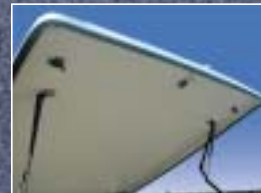
Slam Latch System with cantilever arms and pull-down closure strap
